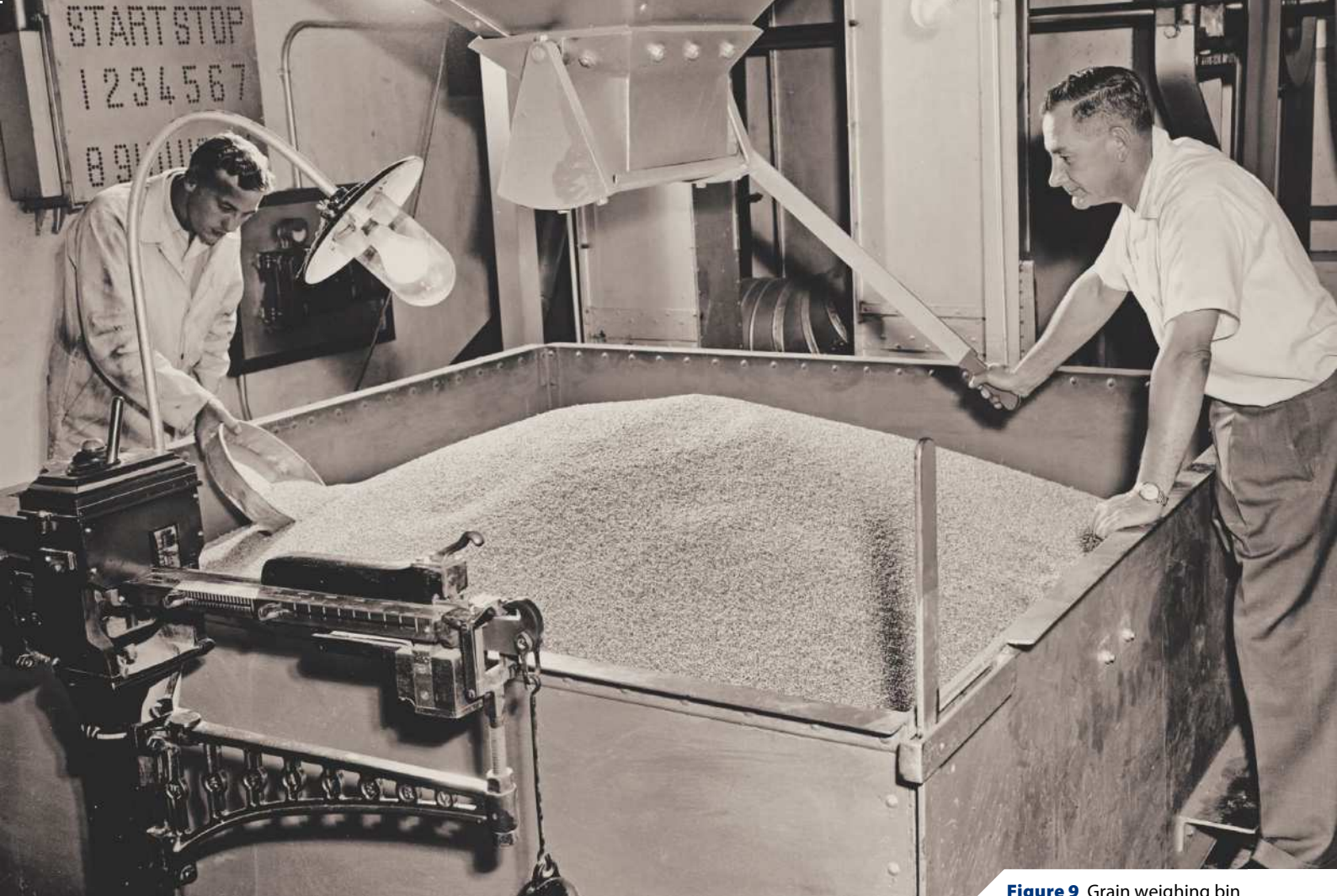
Figure 9 Grain weighing bin
